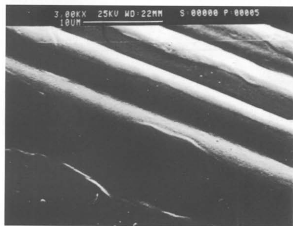
Figure 2 SEM micrographs of T-650/35 carbon fibres before (top) and after (bottom) electrodeposition of polyimide
